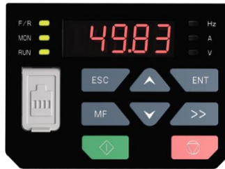
Fig. 4-6 Parameter setting status (b0-02 is set to 49.83Hz)
