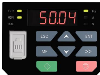
Fig. 4-7 Direct frequency modification status
