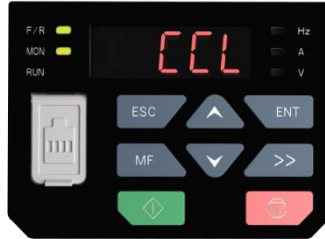
Fig. 4-4 Fault or alarm display status (CCL: Contactor act fault)
