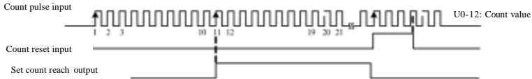
Schematic Diagram for Setting of Set Count Value and Designated Count Value
